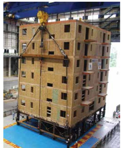
After being lifted to a shake table and subjected to four progressively intense earthquakes, this six-story light-frame building was found to have only minimal damage to the gypsum wallboard and nail connections. (View a video of the test on YouTube.)
