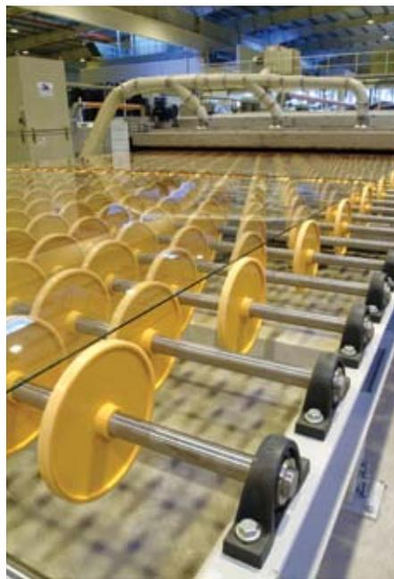
Float glass being rolled along the process line. Glassmaking requires a profound knowledge of physics, chemistry, and related technologies to create a finished product with optimal visual light transmittance, clarity, and integrity for specialized treatments and fabrication.
